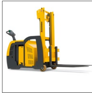
Increased ground clearance with large load wheels.
