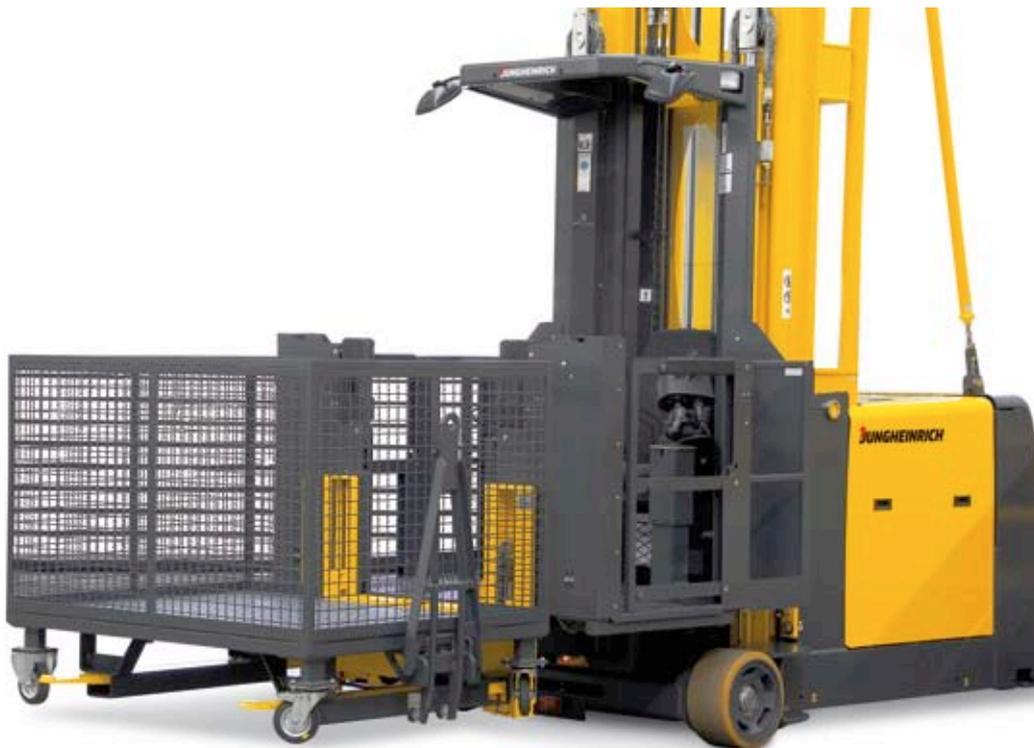
Lower cut out for a picking cage
