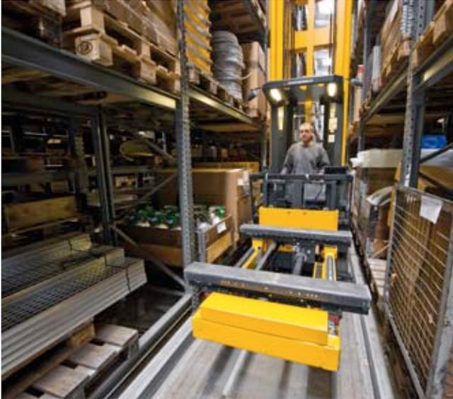
EKX 515, hydraulically adjustable telescopic fork
