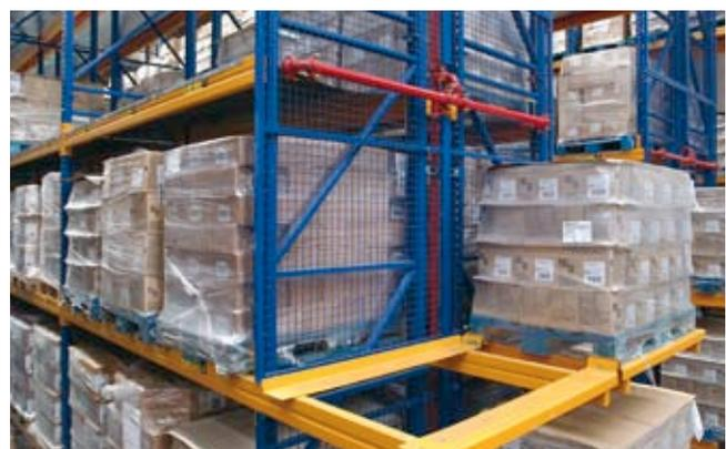
P&D location with projecting bearing surfaces
