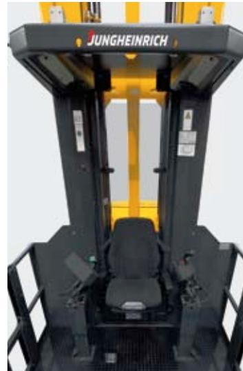
EKX 515, split operator consoles and conversion to a picking truck
