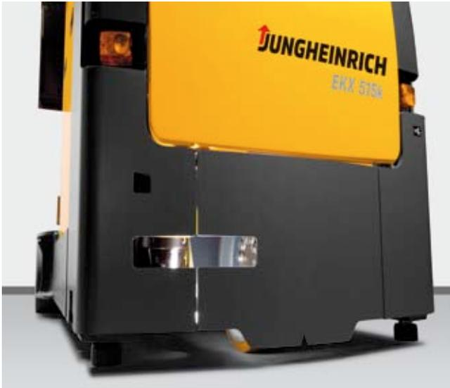
Protected laser scanner in an EKX 515k
