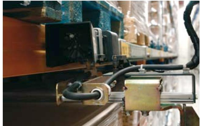
Enclosed conductor rail with current collector
