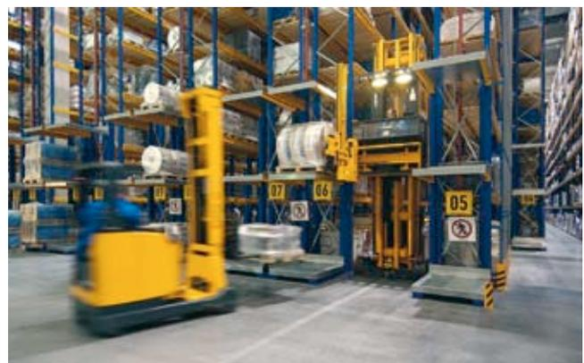
P&D location as separate cantilever type racking
