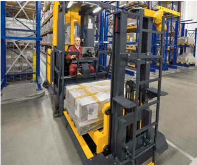
EKX 513, telescopic fork with auxiliary lift in front of the fork and emergency escape ladder
