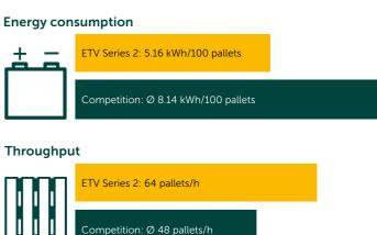
Consumption and transported pallets per hour according to VDI 2198, compared to competition (average value).
